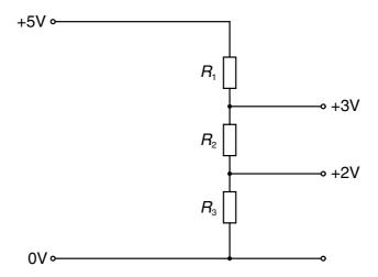
What are possible values for the resistances  $R_1$ ,  $R_2$  and  $R_3$ ?
