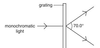
The spacing of the slits in the grating is  $1.00 \times 10^{-6}$  m. The angle between the first order diffraction maxima is  $70.0^{\circ}$ .
