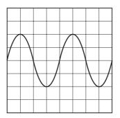
The setting of the time base is then changed from  $10 \,\mathrm{ms}\,\mathrm{cm}^{-1}$  to  $20 \,\mathrm{ms}\,\mathrm{cm}^{-1}$  and the Y-sensitivity is unaltered.
