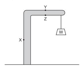
A weight W is lifted by a rope at the end of the beam.
