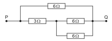
What is the resistance between the points P and Q due to the resistance network?
