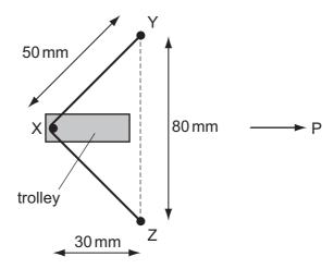
X is at the centre of the elastic and the trolley is to be propelled in the direction P at right angles to YZ. The tension in the elastic is 4 N.
