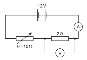
The resistance of the variable resistor is changed from zero to its maximum value.
