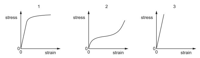
20 The stress-strain graphs for three different materials are shown, not drawn to the same scales.
