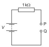
A student attempts to measure the potential difference (p.d.) between points P and Q using two voltmeters, one at a time. The first voltmeter has a resistance of  $1 \text{ k}\Omega$  and the second voltmeter has a resistance of  $1 \text{ M}\Omega$ .
