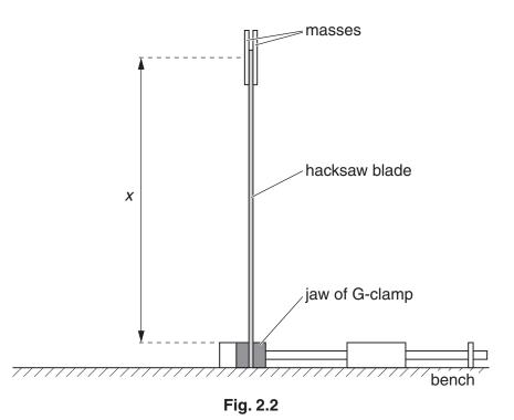
(ii) Measure and record the distance *x* between the top of the jaw of the G-clamp and the centre of the masses, as shown in Fig. 2.2.
