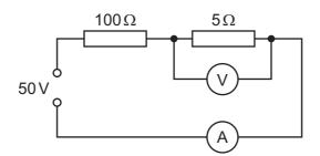
A voltmeter measures the potential difference (p.d.) across the  $5\Omega$  resistor and an ammeter measures the current in the circuit.
