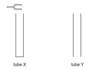
The tubes are identical except tube X is closed at its lower end while tube Y is open at its lower end. Both tubes have open upper ends.
