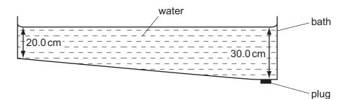
The density of the water is  $1000 \text{ kg m}^{-3}$ .
