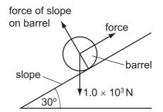
A force is applied to the barrel to move it up the slope at constant speed. The force is parallel to the slope.
