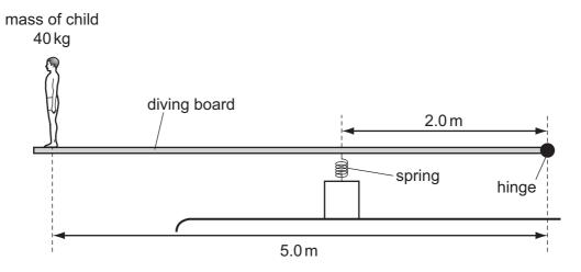
What is the extra compression of the spring caused by the child standing on the end of the board?
