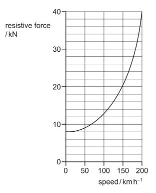
What is the ratio  $\frac{\text{wind resistance}}{\text{wheel friction}}$  at a speed of 200 km h<sup>-1</sup>?
