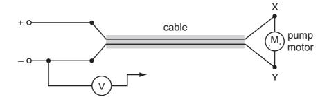
The motor does not work so, to find the fault, the negative terminal of a voltmeter is connected to the negative terminal of the power supply and its other end is connected in turn to terminals X and Y at the motor.
