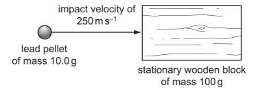
What will be the speed of the block immediately after the pellet is embedded?
