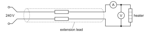
A voltmeter measures the potential difference (p.d.) across the heater as 216 V and an ammeter measures the current through the heater as 7.7 A.
