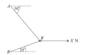
A light inextensible string has its ends attached to two fixed points *A* and *B*, with *A* vertically above *B*. A smooth ring *R*, of mass 0.8 kg, is threaded on the string and is pulled by a horizontal force of magnitude *X* newtons. The sections *AR* and *BR* of the string make angles of 50° and 20° respectively with the horizontal, as shown in the diagram. The ring rests in equilibrium with the string taut. Find
