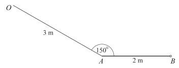
A uniform rod AB, of length 2 m and mass 10 kg, is freely hinged to a fixed point at the end B. A light elastic string, of modulus of elasticity 200 N, has one end attached to the end A of the rod and the other end attached to a fixed point O, which is in the same vertical plane as the rod. The rod is horizontal and in equilibrium, with OA = 3 m and angle  $OAB = 150^{\circ}$  (see diagram). Find
