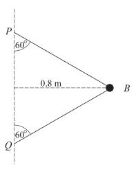
A small ball B of mass 0.5 kg is attached to points P and Q on a fixed vertical axis by two light inextensible strings of equal length. Both of the strings are taut and each is inclined at  $60^{\circ}$  to the vertical, as shown in the diagram. The ball moves with constant speed  $4 \,\mathrm{m \, s}^{-1}$  in a horizontal circle of radius 0.8 m. Find the tension in the string PB.
