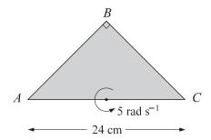
A uniform isosceles triangular lamina ABC is right-angled at B. The length of AC is 24 cm. The lamina rotates in a horizontal plane, about a vertical axis through the mid-point of AC, with angular speed 5 rad s<sup>-1</sup> (see diagram). Find the speed with which the centre of mass of the lamina is moving.
