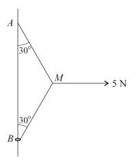
One end of a light inextensible string is attached to a fixed point A of a fixed vertical wire. The other end of the string is attached to a small ring B, of mass  $0.2 \,\mathrm{kg}$ , through which the wire passes. A horizontal force of magnitude 5 N is applied to the mid-point M of the string. The system is in equilibrium with the string taut, with B below A, and with angles ABM and BAM equal to  $30^\circ$  (see diagram).
