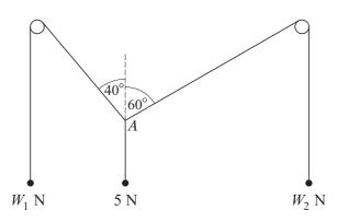
Each of three light strings has a particle attached to one of its ends. The other ends of the strings are tied together at a point A. The strings are in equilibrium with two of them passing over fixed smooth horizontal pegs, and with the particles hanging freely. The weights of the particles, and the angles between the sloping parts of the strings and the vertical, are as shown in the diagram. Find the values of  $W_1$  and  $W_2$ .
