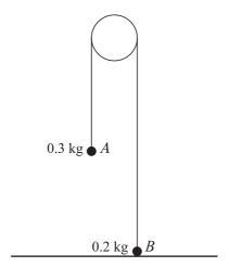
Two particles A and B, of masses 0.3 kg and 0.2 kg respectively, are attached to the ends of a light inextensible string which passes over a smooth fixed pulley. Particle B is held on the horizontal floor and particle A hangs in equilibrium. Particle B is released and each particle starts to move vertically with constant acceleration of magnitude a m s<sup>-2</sup>.
