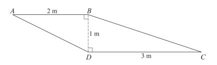
A uniform lamina ABCD is in the form of a trapezium in which AB and DC are parallel and have lengths 2 m and 3 m respectively. BD is perpendicular to the parallel sides and has length 1 m (see diagram).
