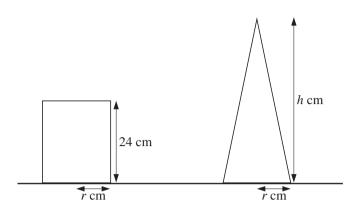
A uniform solid cylinder has height 24 cm and radius r cm. A uniform solid cone has base radius r cm and height h cm. The cylinder and the cone are both placed with their axes vertical on a rough horizontal plane (see diagram, which shows cross-sections of the solids). The plane is slowly tilted and both solids remain in equilibrium until the angle of inclination of the plane reaches  $\alpha^{\circ}$ , when both solids topple simultaneously.
