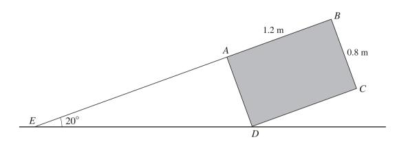
ABCD is a central cross-section of a uniform rectangular block of mass 35 kg. The lengths of AB and BC are 1.2 m and 0.8 m respectively. The block is held in equilibrium by a rope, one end of which is attached to the point E of a rough horizontal floor. The other end of the rope is attached to the block at A. The rope is in the same vertical plane as ABCD, and EAB is a straight line making an angle of  $20^{\circ}$  with the horizontal (see diagram).
