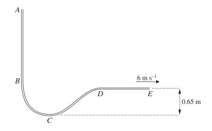
A smooth narrow tube AE has two straight parts, AB and DE, and a curved part BCD. The part AB is vertical with A above B, and DE is horizontal. C is the lowest point of the tube and is 0.65 m below the level of DE. A particle is released from rest at A and travels through the tube, leaving it at E with speed 6 m s<sup>-1</sup> (see diagram). Find
