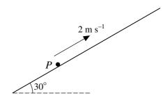
A particle P of mass 0.2 kg is projected with velocity  $2 \,\mathrm{m \, s^{-1}}$  upwards along a line of greatest slope on a plane inclined at 30° to the horizontal (see diagram). Air resistance of magnitude  $0.5 \,\mathrm{v}$  N opposes the motion of P, where  $\mathrm{v \, m \, s^{-1}}$  is the velocity of P at time t s after projection. The coefficient of friction between P and the plane is  $\frac{1}{2 \,\sqrt{3}}$ . The particle P reaches a position of instantaneous rest when t = T.
