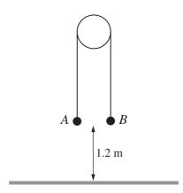
Particles A of mass 0.4 kg and B of mass 1.6 kg are attached to the ends of a light inextensible string which passes over a fixed smooth pulley. A is held at rest and B hangs freely, with both straight parts of the string vertical and both particles at a height of 1.2 m above the floor (see diagram). A is released and both particles start to move.
