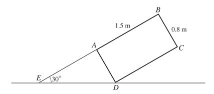
ABCD is the cross-section through the centre of mass of a uniform rectangular block of weight 260 N. The lengths AB and BC are 1.5 m and 0.8 m respectively. The block rests in equilibrium with the point D on a rough horizontal floor. Equilibrium is maintained by a light rope attached to the point A on the block and the point E on the floor. The points E, E0 and E1 lie in a straight line inclined at 30° to the horizontal (see diagram).
