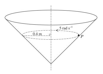
A particle *P* of mass 0.5 kg moves in a horizontal circle on the smooth inner surface of a hollow cone which is fixed with its axis vertical and its vertex downwards. *P* moves with angular speed  $5 \text{ rad s}^{-1}$  in a circle of radius 0.4 m (see diagram). Show that the semi-vertical angle of the cone is  $45^{\circ}$  and calculate the magnitude of the force exerted on *P* by the surface of the cone. [6]
