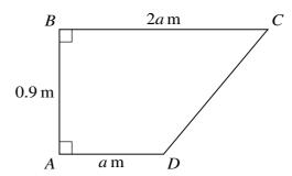
The diagram shows the cross-section ABCD through the centre of mass of a uniform solid prism. AB = 0.9 m, BC = 2a m, AD = a m and angle  $ABC = \text{angle } BAD = 90^{\circ}$ .
