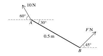
A non-uniform rod AB of length 0.5 m is freely hinged to a fixed point at A. The rod is in equilibrium at an angle of 30° with the horizontal with B below the level of A. Equilibrium is maintained by a force of magnitude F N applied at B acting at 45° above the horizontal in the vertical plane containing AB. The force exerted by the hinge on the rod has magnitude 10 N and acts at an angle of 60° above the horizontal (see diagram).
