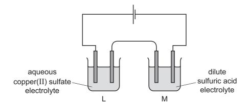
Which row shows what happens to the concentration of the electrolyte in L and in M as the electrolysis proceeds?
