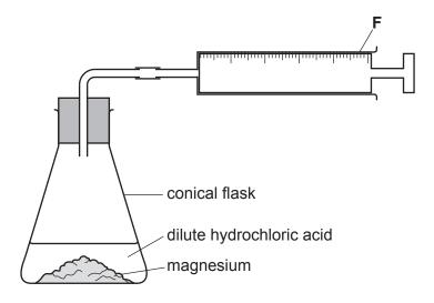
In each experiment the student adds dilute hydrochloric acid to magnesium. The volume of hydrogen in apparatus **F** is recorded every 30 seconds.
